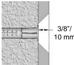
The anchor must be sunk at least 3/8"/10 mm into the plaster coating.
